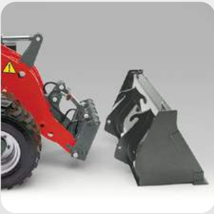
Efficient change of attachments. Thanks to the hydraulic quickhitch system, attachments can be comfortably and quickly exchanged. A good view of the quickhitch plate makes the changeover of attachments particularly easy. With the 2-hand operation when uncoupling, changing over the attachments is expressly safe and the machine is immediately ready to use again.
