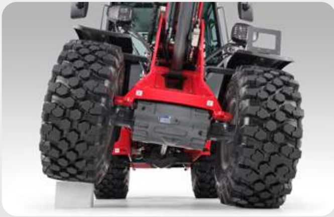
Maximum traction due to the articulated pendulum joint. With the articulated pendulum joint, all four wheels maintain ground contact, even on uneven terrain. This increases the machine's productivity and provides the operator with optimal control. Front and rear carriages can be oscillated independently of one another. This way the operator can react with precision to any imperfection. This increases comfort and creates a safe driving experience.
